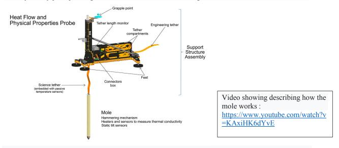
It is a heat flow sensor which aims to measure the heat given off by the Martian subsoil. The mole had to sink to a depth of 5 meters in order to take measurements without being disturbed by daily and seasonal variations in surface temperature.
