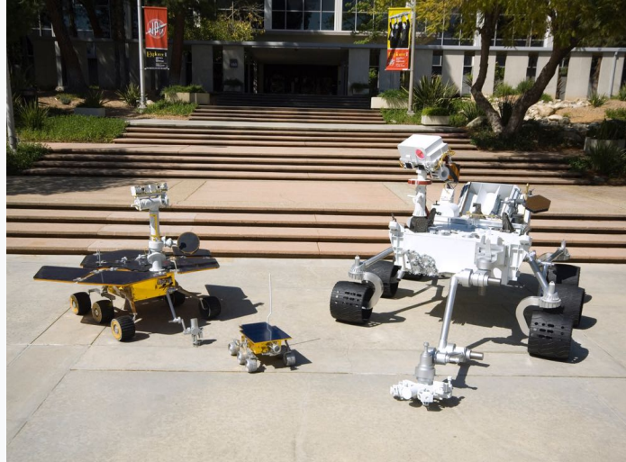
Models of NASA Mars rovers. From left to right: Mars Exploration Rover, Sojourner and Curiosity.
